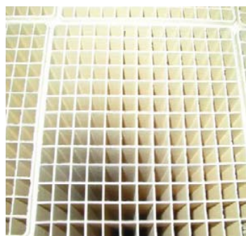
Figure 1.67: Example of an individual catalyst used for the SCR technique [140, Italy, 2007]
