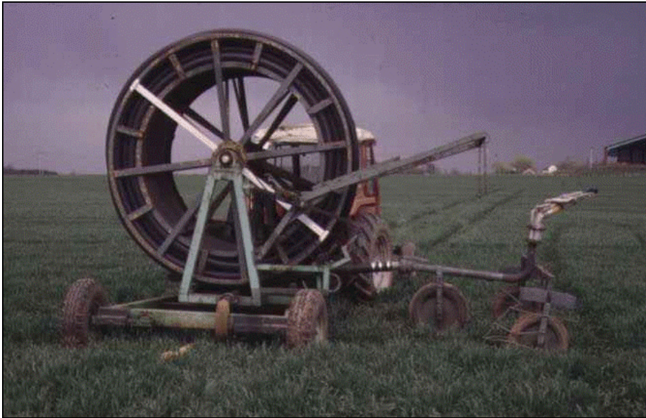
Figure 2.37: Example of a raingun [220, UK, 2002]
